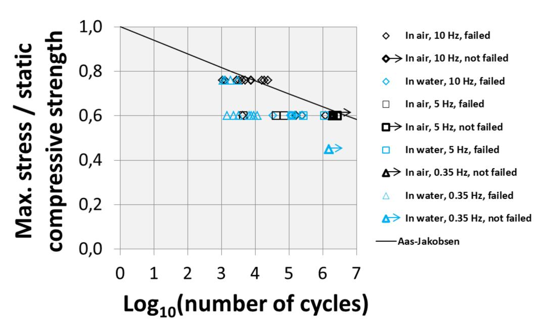
However, the specimens tested in water (shown in blue colour) exhibit markedly lower fatigue strengths. This can also be seen in the succeeding figure showing the fatigue results at the 60% maximum stress level. At all frequencies, testing in water led to lower fatigue strengths than in air, where several of the specimens in each series survived more than 2 million cycles.
