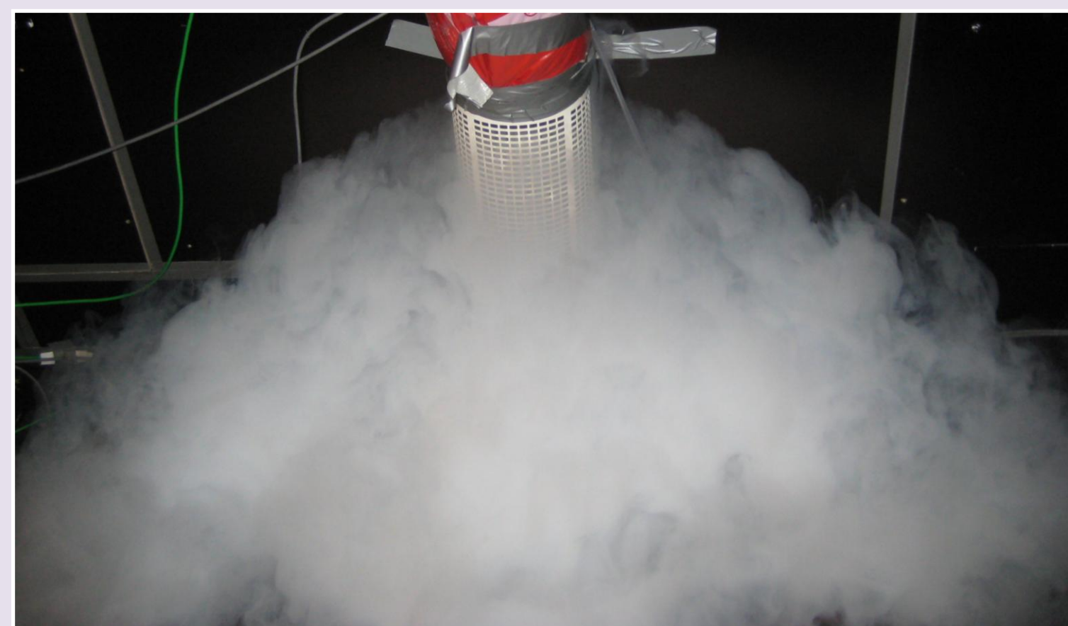
Diffuser 1. (a) Smoke visualization of the stratified flow generated by the cold supply air, which is common with a wall-mounted displacement diffuser. (b) Velocity measurements along the horizontal line.
