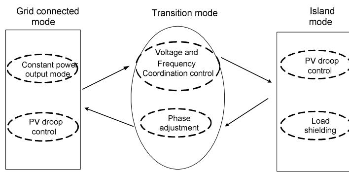
Fig5The operation modes and their transition of micro-grid
