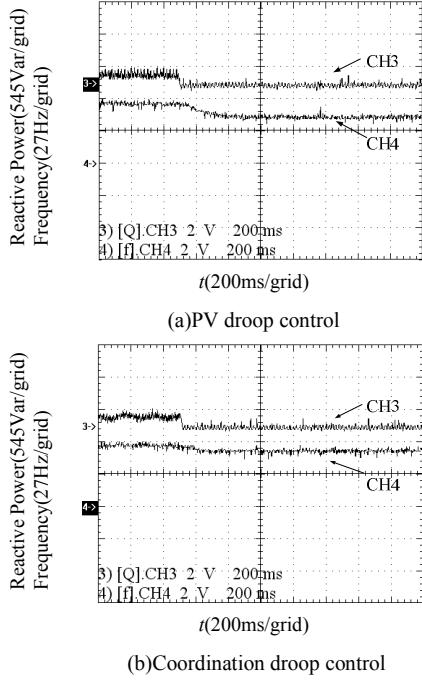
Fig.14The output reactive power and the frequency of inverter while disconnecting to grid
