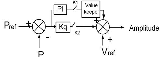
Fig 3 Voltage reference compensation in opposite droop control
