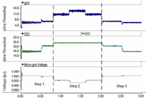
Fig9 the transition between droop control and constant power output mode
