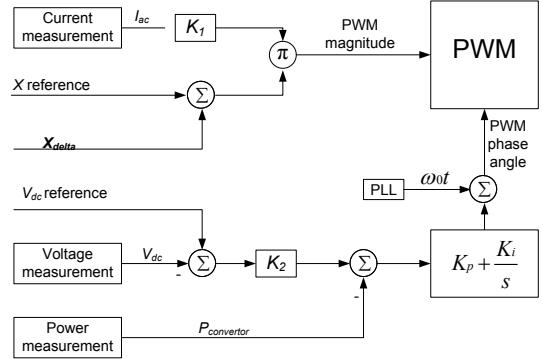
Fig.2. SSSC voltage regulator scheme
