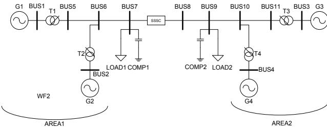
Fig.6. Four-machine two-area test system
