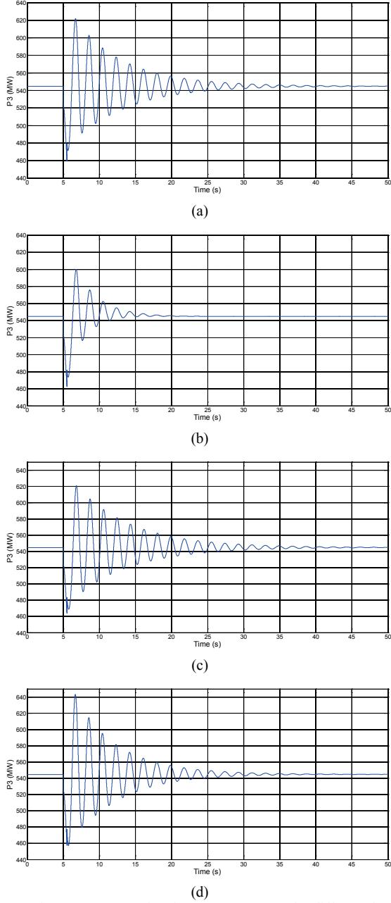
Fig.7. Active power generation from generator 3 under different damping conditions: (a) no damping controller; (b) input  $\Delta\omega_{r3}$  parameter PARA1; (c) input  $\Delta\omega_{rl}$  parameter PARA1; (D) input  $\Delta\omega_{rl}$  parameter PARA2
