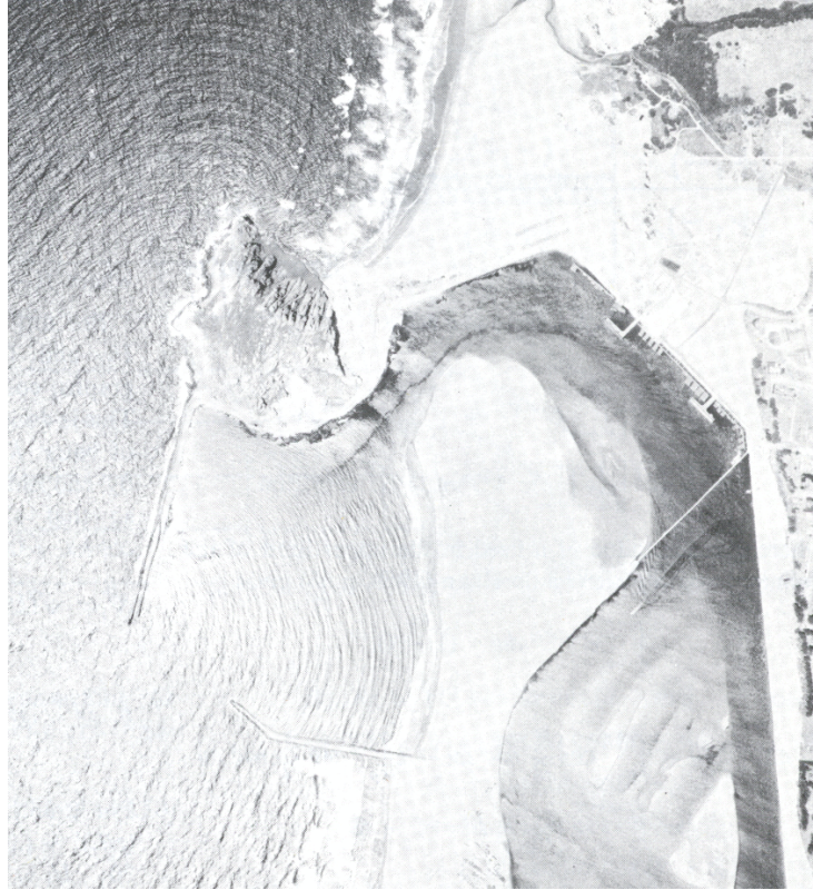
Figure 4.8: Diffraction around breakwater head.
