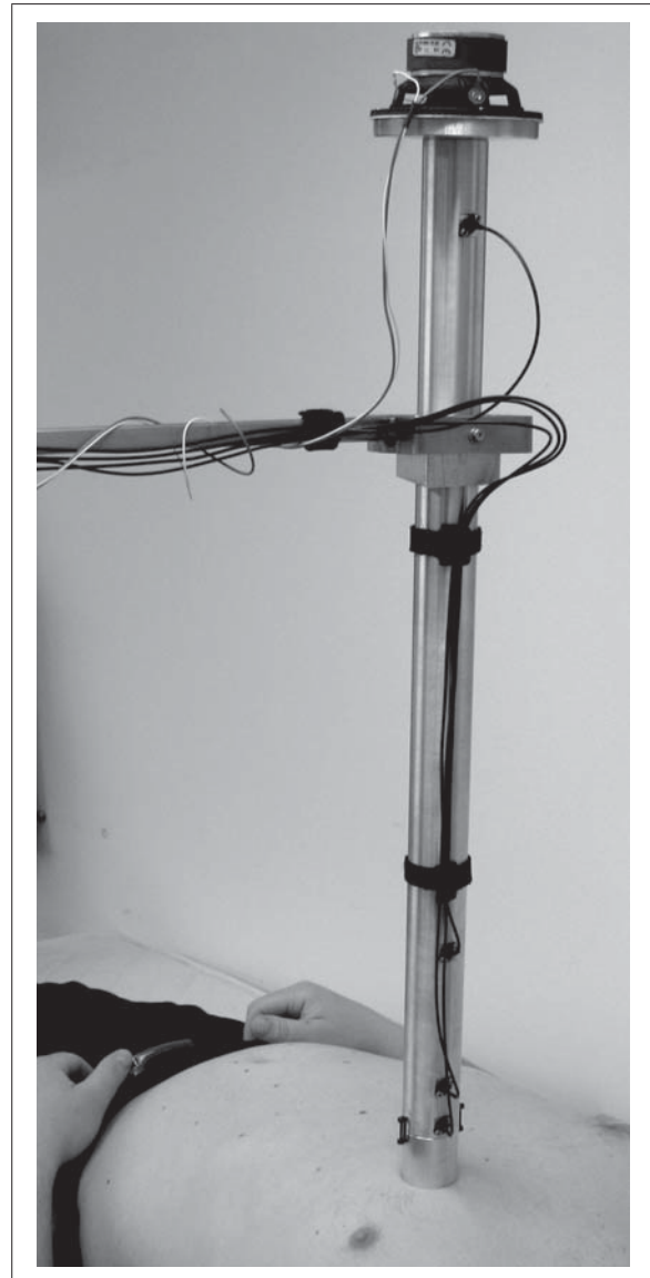
Figure 2. Impedance tube positioned on chest. The gyroscopic support insures a perpendicular angle to the chest.
