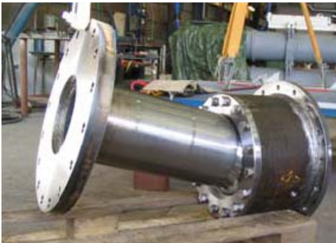
Figure 10: Manufactured joint and fitting on main platform.
