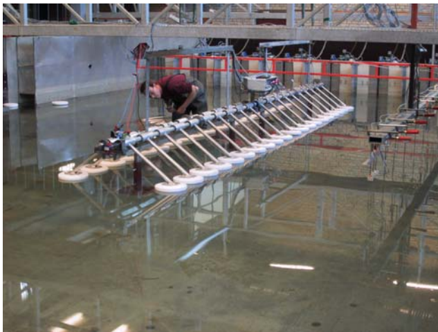
Fig. 5: The Wave Star Nissum Bredning 1:10 scale prototype (upper). Wave Star model in wave tank (left), and prototype in storm safe mode (right).
