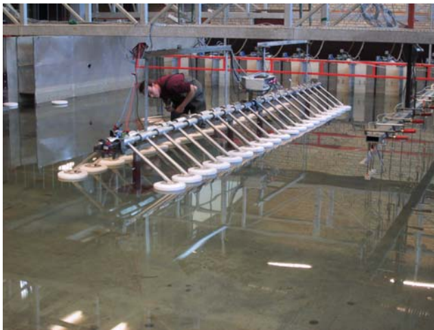
Fig. 5: The Wave Star Nissum Bredning 1:10 scale prototype (upper). Wave Star model in wave tank (left), and prototype in storm safe model (right).
