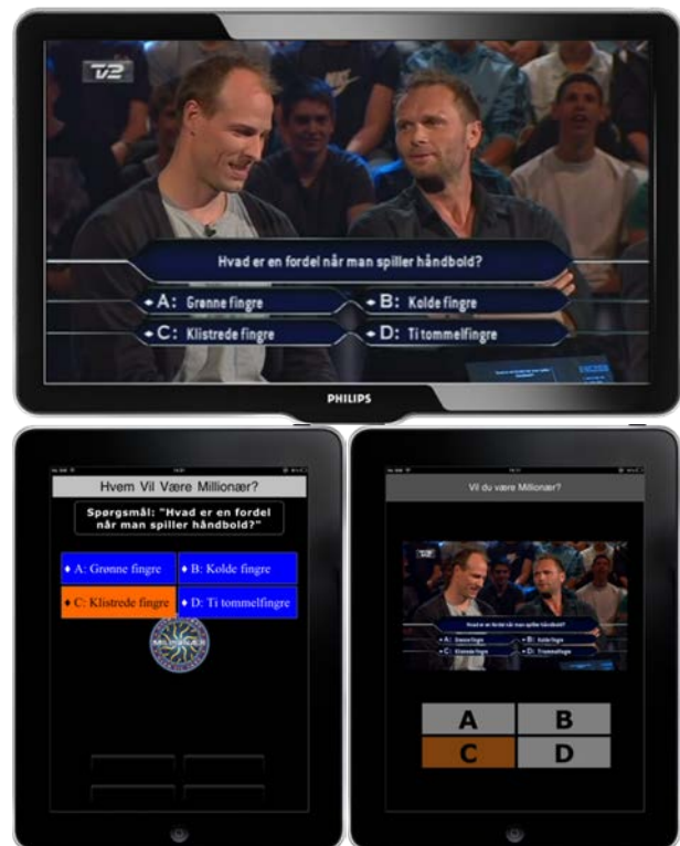
Figure 1. Prototype illustrating separation of content and control: The live program plays on the TV (top), while the second screen displays either the interactive functions alone (bottom left), or with the video stream (bottom right).
