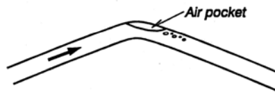
Figure 2.5. Air pocket at a high point.
