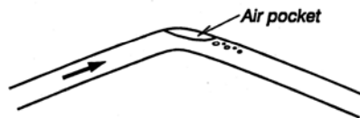
Figure 2.5. Air pocket at a high point.
