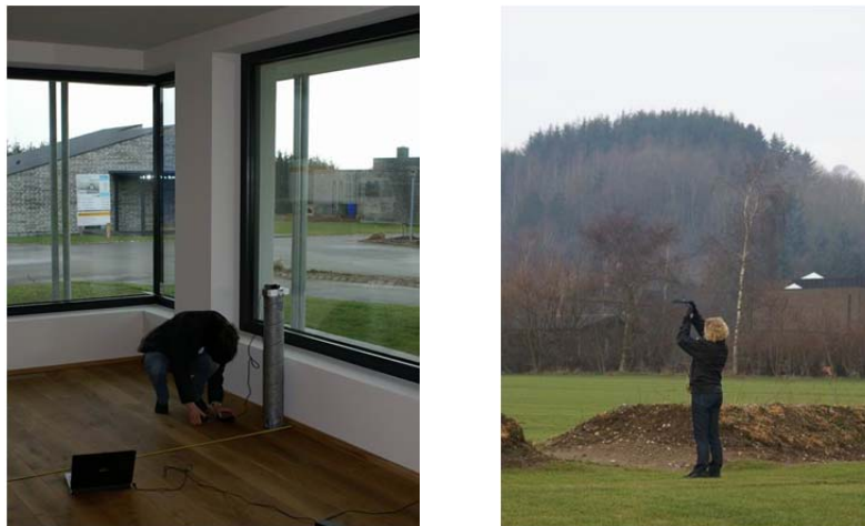
Figure C.1. Measuring the daylight in the Comfort Houses.
