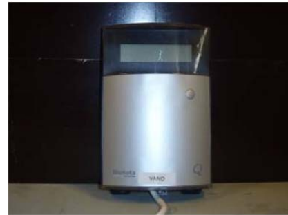
Figure B.0.4: HGQ1 heat consumption measurer.
