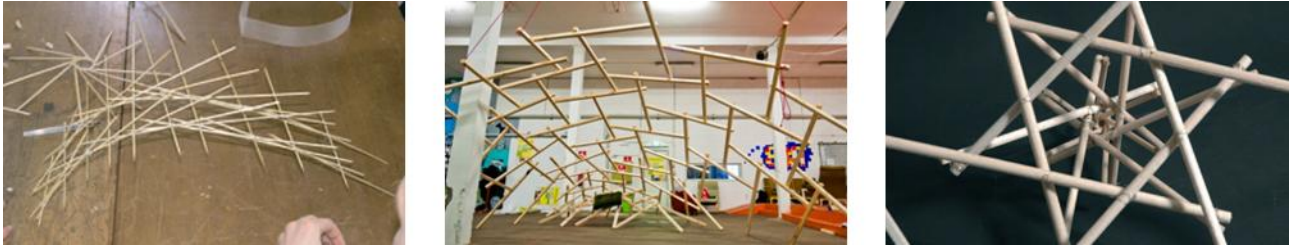
Figure 1: Left, 1D reciprocal bridge inspired by the Leonardo's bridge; Middle, 2D reciprocal roof with fans composed by four elements; Right: 3D conceptual reciprocal structure by Popovic Larsen.
