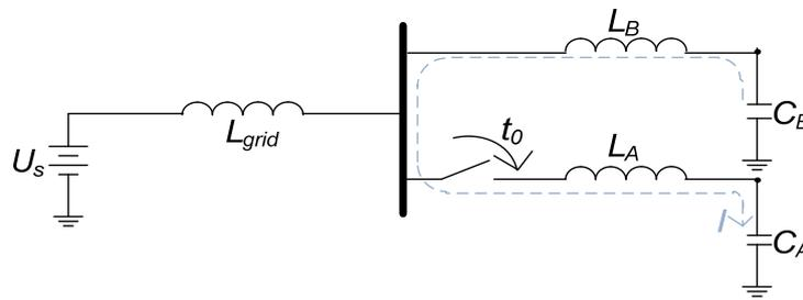
The situation is different when no cables are connected to the bus bar, as cable A will interact with the external network as shown in Figure 11.
