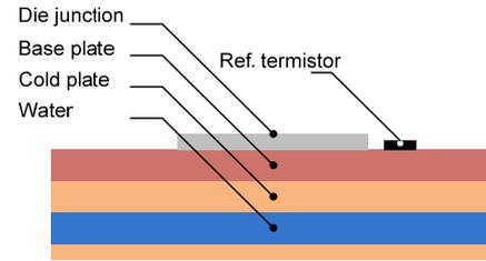
**Figure 2:** Material layers in the thermal resistance network of Luminus CBT90 diode and cold plate.
