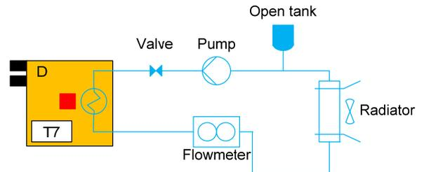
**Figure 6:** Schematic view of water cooling circuit.
