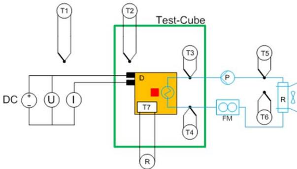
**Figure 7: Experimental setup used in cold plate experiments.**
