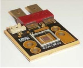
**Figure 3:** Red Luminus CBT90 LED diode.
