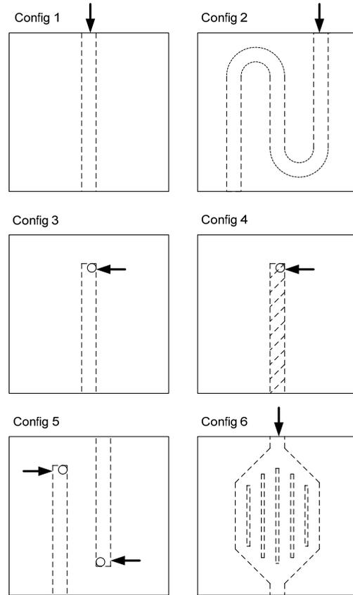
**Figure 4:** Cold plate designs. The arrow indicates the fluid inlet to the cold plate. The cold plates given in configuration 3-5 utilize tangential inlet to the cooling channel.
