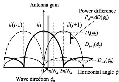
Figure 1. Three overlapping radiation patterns of the array.
