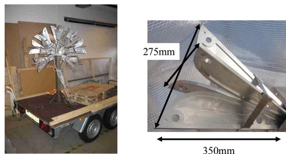
Figure 2. Horn antenna array and antenna probe.
