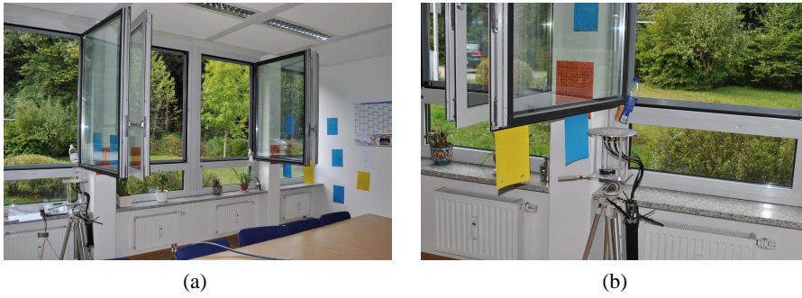
Figure 5.5: (a) The receiver is at position Rp1 and W1 to W4 are open. (b) The receiver at position Rp2. The metallic frame of W1 is only approximately 10 cm above the antenna array.
