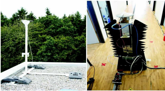
Fig. 1. Left plot: transmit antenna located on the rooftop; Right plot: model train including mounted receive antenna
