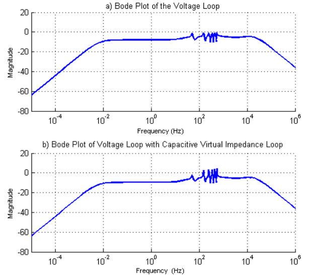
Fig. 5. a) Bode plot of the closed loop transfer function  $\frac{V_c(s)}{V_{ref}(s)}$  without the virtual impedance loop for the PR controller parameters given in Table II. b) Bode plot of the closed loop transfer function  $\frac{V_c(s)}{V_{ref}(s)}$  with the virtual impedance loop for the PR controller parameters given in Table II.
