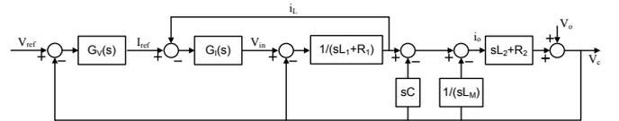
Fig. 3. Block diagram of the inner loops. The plant consists of an LC filter and an isolation transformer to interface with the microgrid.  $L_M$ ,  $L_2$  and  $R_2$  are the transformer parameters namely the magnetization inductance, leakage inductance and winding resistance.  $G_V(s)$  and  $G_I(s)$  are the voltage and current controller transfer functions respectively.
