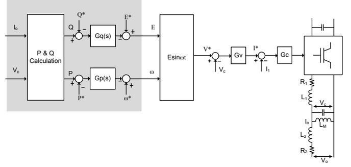
Fig. 2. Microsource Inverter control block diagram for islaned mode.
