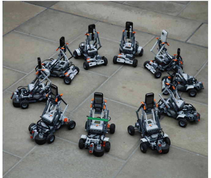
Figure 2. LEGO robots carrying 10 Nokia mobile phones
