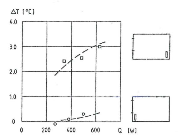
Fig. 1. Temperature difference between the height y = 1.8 m and y = 0.05 m at different loads and locations of radiator. From /2/.
