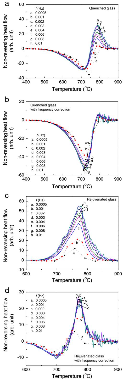
Fig. 3. The non-reversing heat flow at modulation frequencies ( $f$ ) from 0.0005 to 0.01 Hz: (a) quenched glass; (b) quenched glass with  $f$  correction; (c) rejuvenated glass; (d) rejuvenated glass with  $f$  correction.
