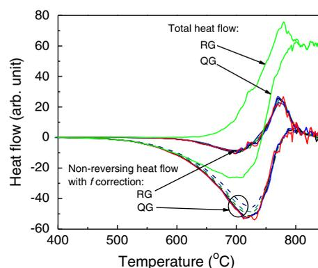
Fig. 5. The area enclosed by the non-reversing heat flow master curves of quenched glass (QG) and rejuvenated glass (RG) for frequencies ( $f$ ): 0.002, 0.003, 0.004, 0.006, 0.008, 0.01 Hz, comparing with the area enclosed by the total heat flow curves of QG and RG.
