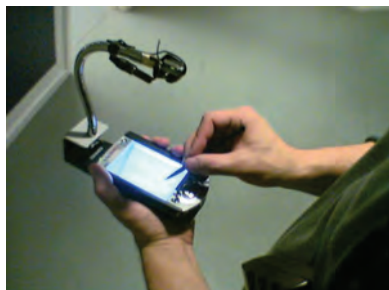
Figure 14. Wireless camera mounted on PDA
