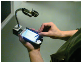
Figure 8. Wireless miniature camera mounted on PDA
