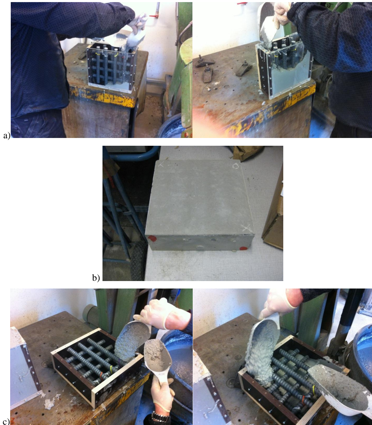
Figure 8 – Casting of the UHPFRC samples with FiReP® reinforcement (AAU, spring 2012): a) 2 point casting of a vertical sample; b) finished vertical sample cast vertically from 2 points (shown in red); c) 2 point casting of a horizontal sample.
