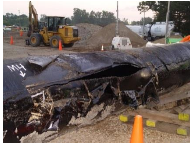
Figure 1 .Failure because of high pressure
