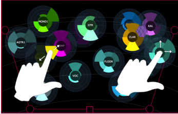
Figure 2: Overview of the main stage. Widgets represent audio channels, which are positioned in relation to the listening position represented by the pink square in the bottom centre. The distance from the listening position determines the volume of the corresponding audio channel. The angle determines the panning.
