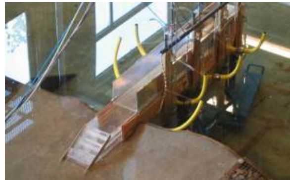
Figure 9: Model for 3D overtopping tests.
