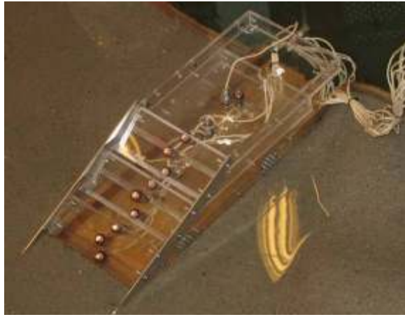
Figure 2: SSG caisson model.
