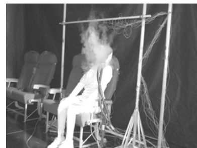
Figure 2. Effectiveness and experiment with smoke visualization for the neck supporter.
