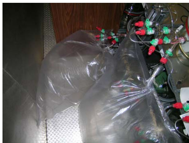
Figure 5. Sampling procedure at the exhaust of the emission chamber (20l chamber).
