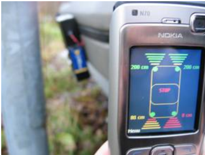
Fig. 7. A picture taken during the tests of the parksensor application. On the screen of the phone, the colored bars indicate the distance measurements coming from the four sensors placed on the car.
