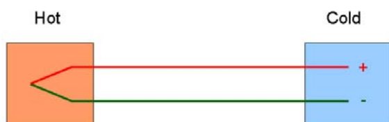
Figure 1. Functional principle of thermocouples
