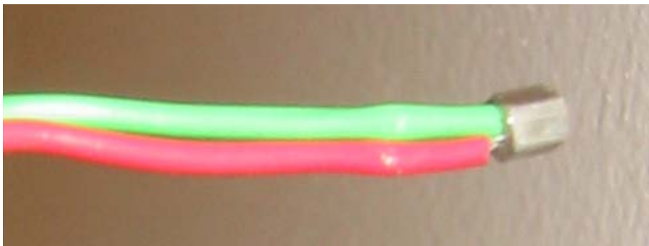
Figure 2. Thermocouple with aluminium tip.
