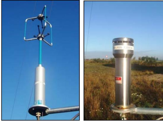
Figure 44. The 3D (left) and 2D(right) ultrasonic anemometer.
