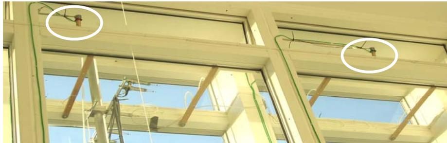
Figure 34. Measurement of outlet air temperature from the DSF.
