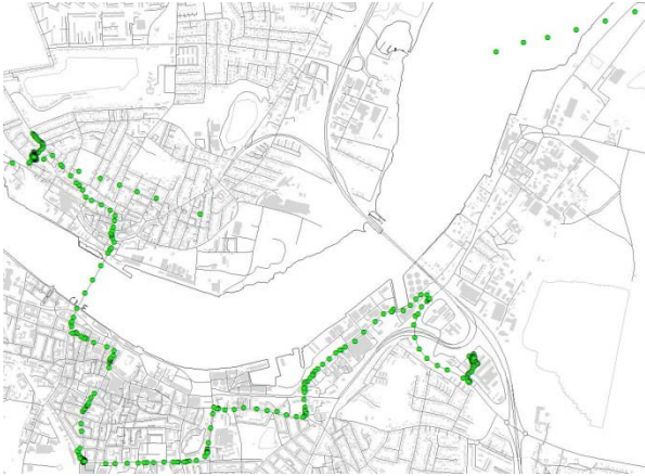
2 An example of a trip affected by Scatter type 2. During the point recording process, the receiver lost track and registered points in a linear pattern in the upper right corner.
