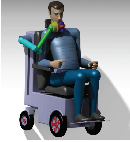
Figure 1: A light-weight anthropomorphic robotic arm mounted on an electric wheelchair.
