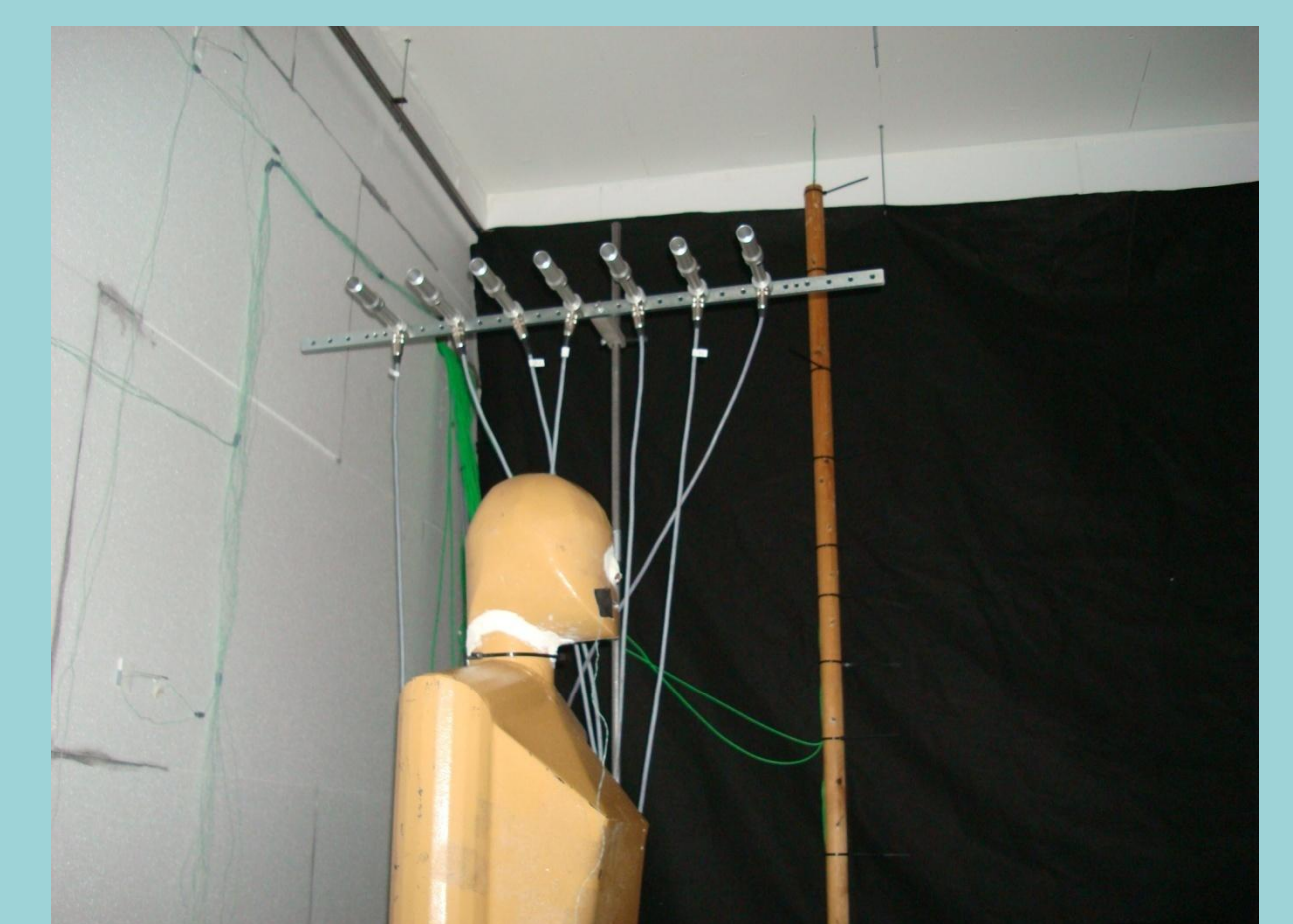
Breathing thermal manikin and location of sensors
