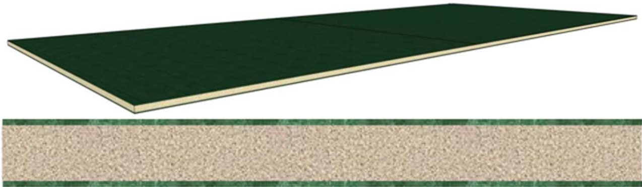
Figure 2.4: Illustration of a carbon FRP composite panel (top) and a close-up on the core and the fibre reinforced laminates (bottom). (Evegren and Rahm 2012, p 11)
