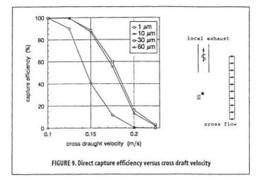
that the flow of shielding gas in gas-metal-arc welding enhanced the spread of generated welding fumes and deteriorated capture efficiency of the local exhaust system under investigation.
