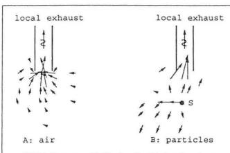
FIGURE 3. Flow pattern of air (A) and particles (B) in front of an exhaust opening at a location with a slight cross draft (redrawn from calculated data). 60 µm particles of unit density are emitted with an initial velocity.
