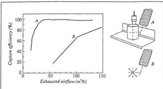
FIGURE 1. Capture efficiency versus exhausted airflow of a local exhaust at a can filling machine (A) and a simple point source (B). The distances are identical from the exhaust openings to center of the can and the point source, respectively. Tracer gas is used as a simulated contaminant for measuring local exhaust capture efficiency. Madsen and Tveit.<sup>(1)</sup>
