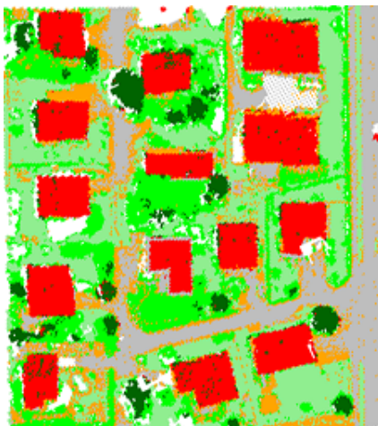
Figure 5. Land cover map (‘raw’ result). Six classes are coded by colours. (red=“building”, light green=“grass”, dark green=“tree”, green=“hedge&bush”, grey=“road & parking lot”, orange=“wall & car port”)
