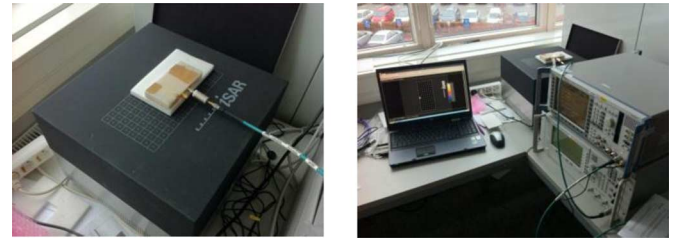
Fig. 18. The measurement setup of iSAR system.
