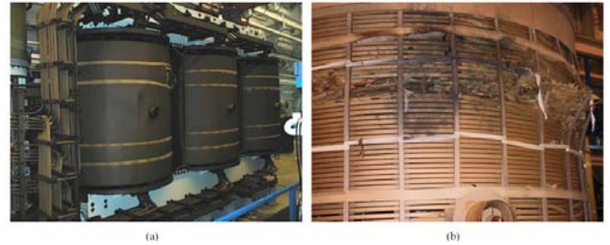
Fig. 7. The damaged transformer, a) The three phases with the faulty phase furthest to the left. b) The faulty winding seen from the outside after various paper layers have been removed.
