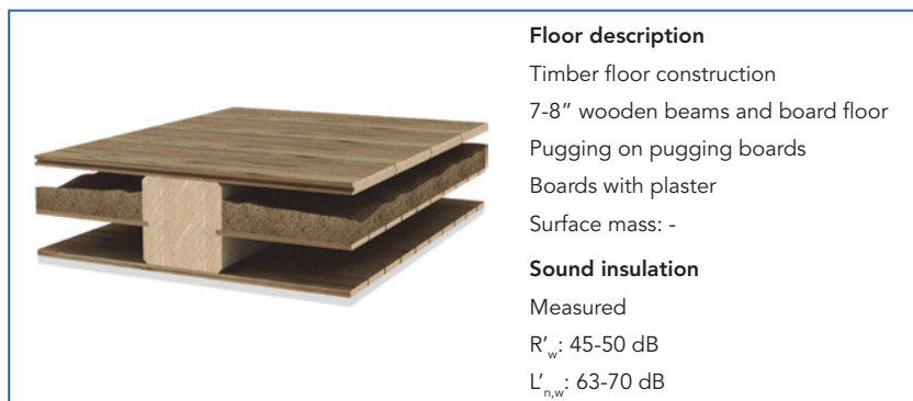
Figure 5.18. Floor performance in building type commonly used up to 1950. Drawing from [9], [15].
