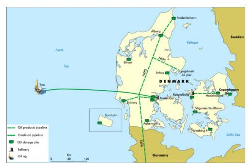
Figure 8. Oil products pipeline system [55]
