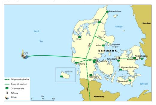
Figure 8. Oil products pipeline system [55]
