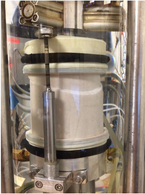
Figure 14. Illustration of failure in extension of test no. 3.
