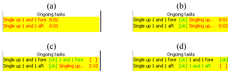
Fig. 9. Sequence of commands being executed, confirmed, completed and confirmed
