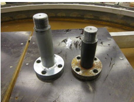
Figure 35: Transition piece 1 (to the left) is used when conducting CPTs. Transition piece 2 (to the right) is used when installing or uninstalling the pile.
