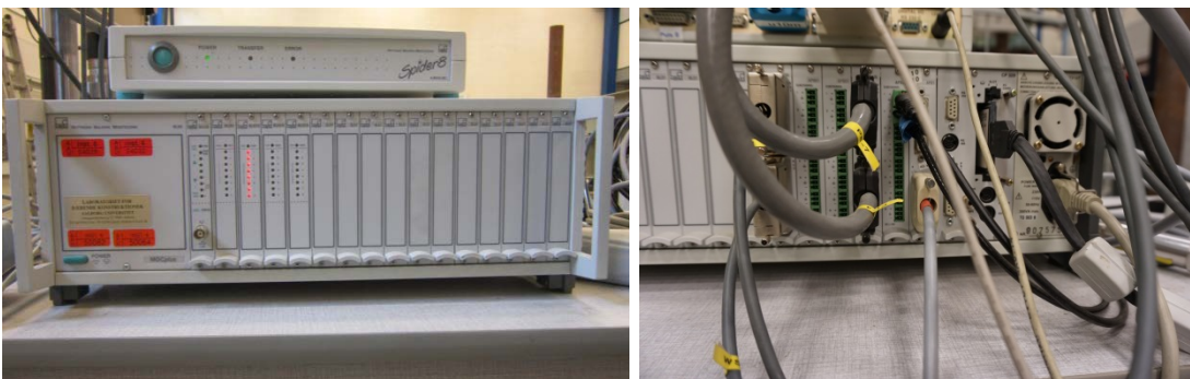
Figure 12: Left: Front of MGCplus. Right: the pore pressure transducers, the air pressure transducer, the membrane pressure transducer, the real pile head displacement and the load and displacement recorded by MOOG connected to MGCplus.
