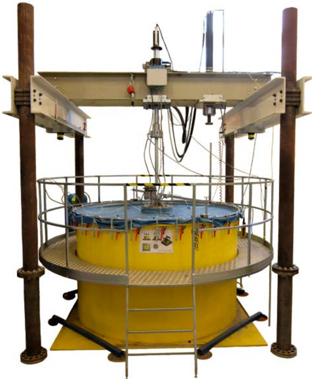
Figure 1: Test setup with applied suction.
