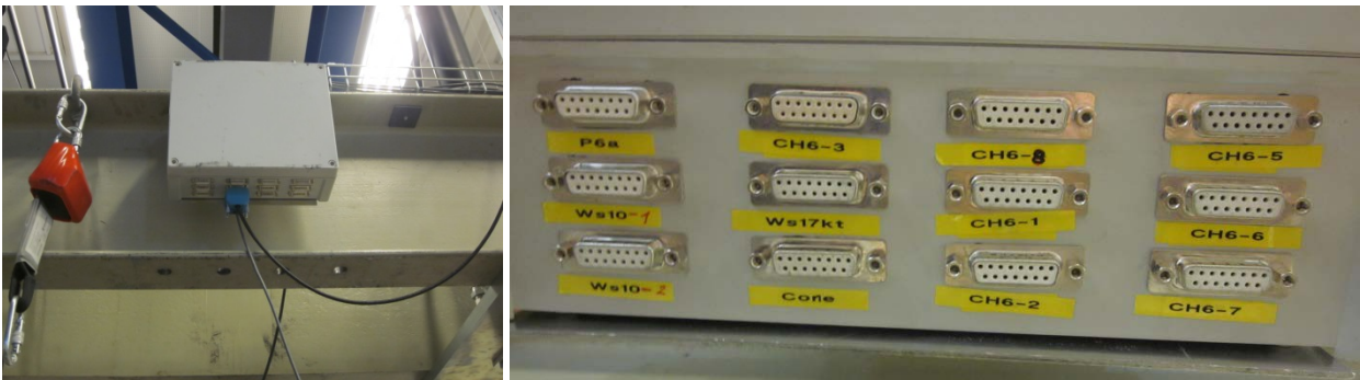
Figure 11: The CPT device is connected to Spider8 through the box on the load frame through the socket "Cone" and the displacement transducer is connected via the socket "WS17kt".
