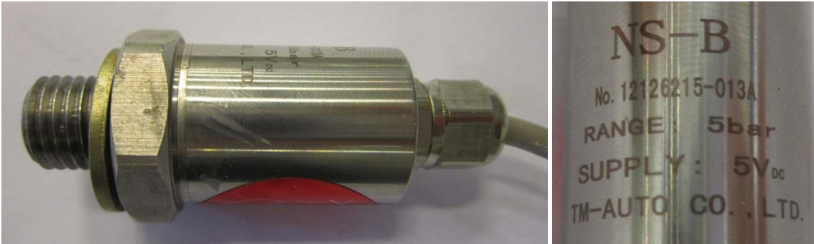
Figure 31: Example of pore pressure transducer.
