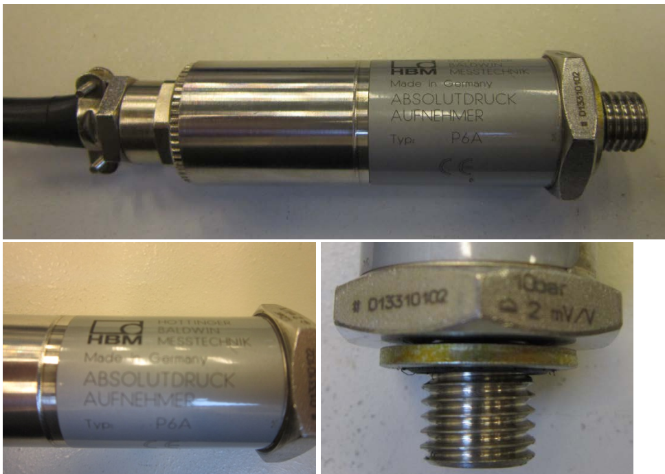
Figure 32: Air pressure transducer.
