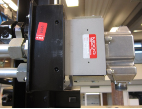
Figure 27: Displacement transducer for Hydraulic cylinder 2.
