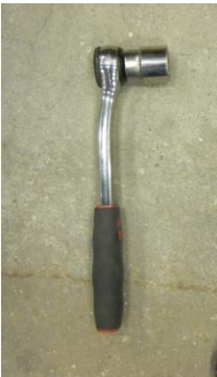
Figure 42: Ratchet for connecting the pile and the CPT to the transition pieces and for tightening the rig with Hydraulic piston 1 to the load beam when conducting CPTs.
