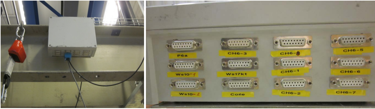
Figure 13: The displacement transducers are connected to MGCplus via the sockets “WS10-1” and “WS10-2”. The pore pressure transducers are connected through CH6-1, CH6-2, CH6-5, CH6-6 and CH6-7. The membrane pressure transducer is connected to MGCplus via CH6-8.
