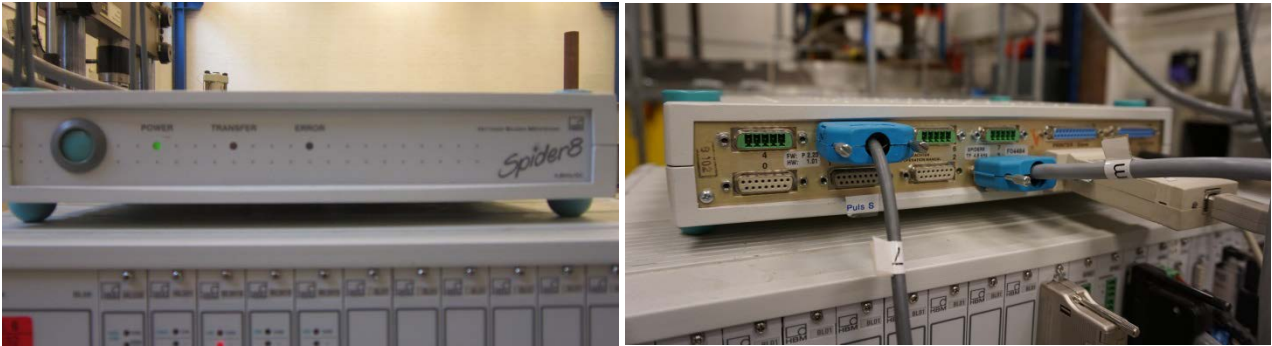
Figure 10: Left: Front of Spider8. Right: CPT device, Load cell 1 and displacement transducer connected to Spider8
