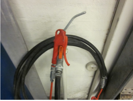
Figure 40: Compressor for cleaning the pore pressure pipes and the sand box edge.
