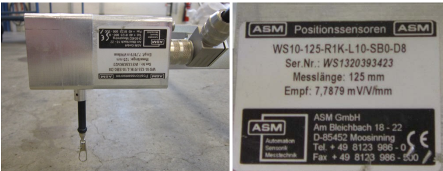
Figure 29: Displacement transducer WS10-1.
