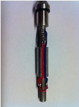
Figure 18: Strain gauges and wiring inside the CPT to measure the cone resistance.
