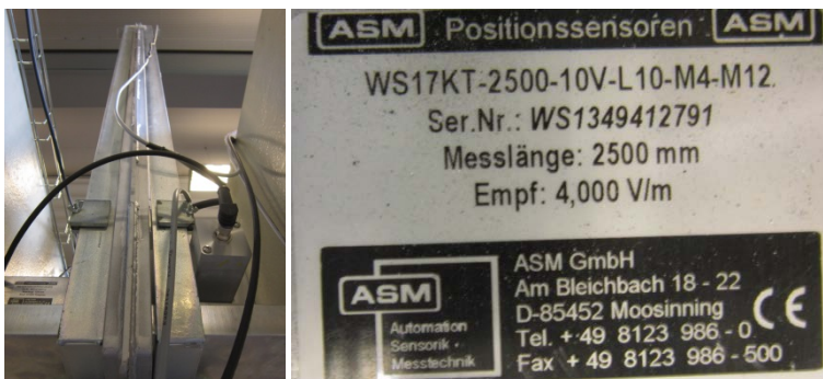
Figure 24: Displacement transducer for hydraulic cylinder 1.
