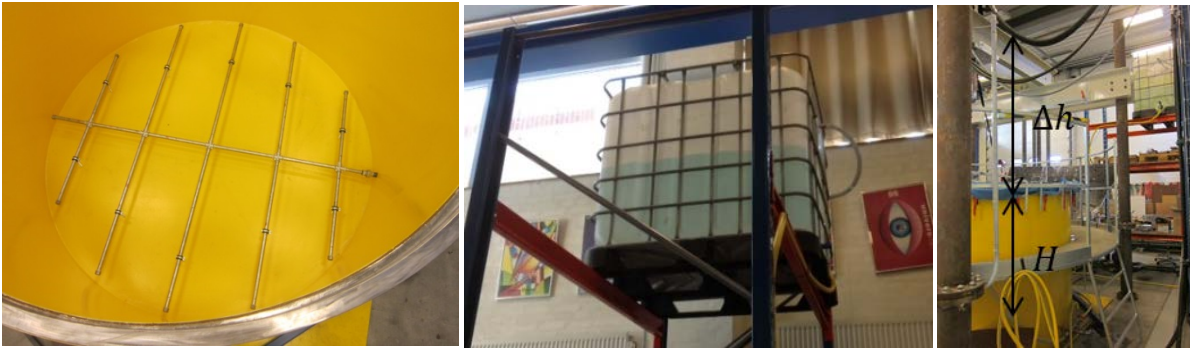
Figure 3: The drainage pipes in the bottom of the sand box. The water tank. The ascension pipe.
