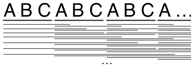
Fig. 11.8 Closed patterns found in a cyclic sequence of symbols. The occurrences of the pattern shown in thick lines do not overlap, whereas those shown in thin lines do
