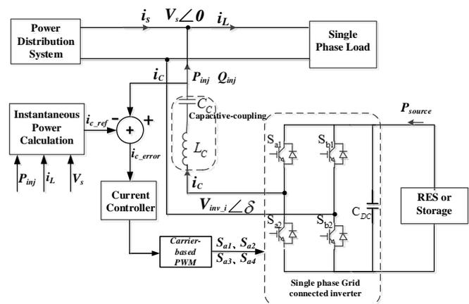
Fig. 1 System configuration of a single-phase CGCI
