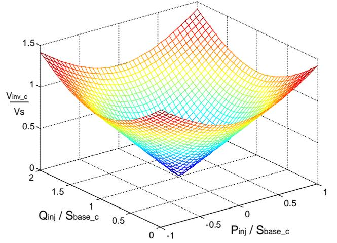
Fig. 2 Variation in inverter voltage with power
