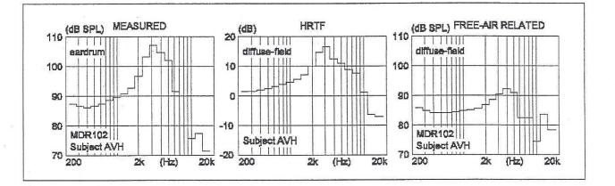
Figure 1. Example of derivation of diffuse-field related third-octave spectrum from eardrum measurements. Left frame: Spectrum at eardrum. Center frame: Diffuse-field eardrum HRTF. Right frame: Diffuse-field related spectrum. A-weighting and summation gives a diffuse-field related sound pressure level of 99.5 dB(A). Sony MDR102 headphone supplied with pink noise (500 mV 20-20,000 Hz). Subject AVH left ear.
