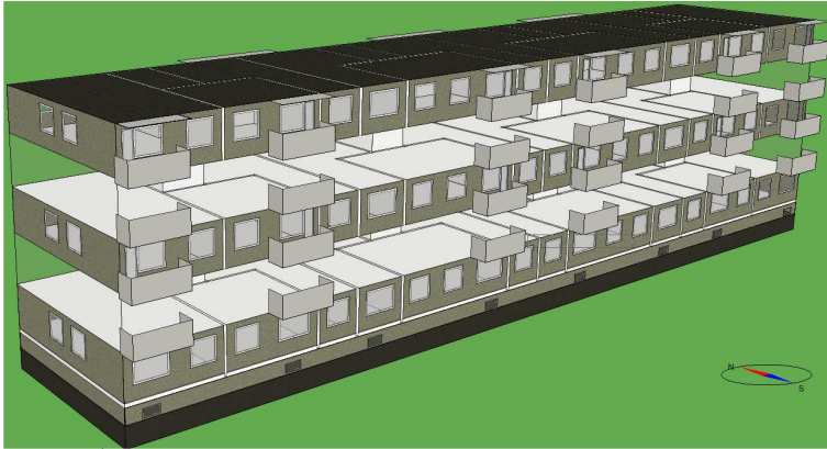
Fig. 1 The model of a typical 5-story concrete large-panel apartment building built in 1960-1980. The middle floor results have been multiplied by 3.
