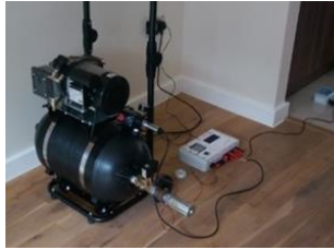
Fig 2 Device for air-pulse test in development
