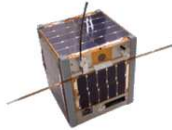
Figure 2. The XI-IV Cubesat to be deployed from SSETI-Express
