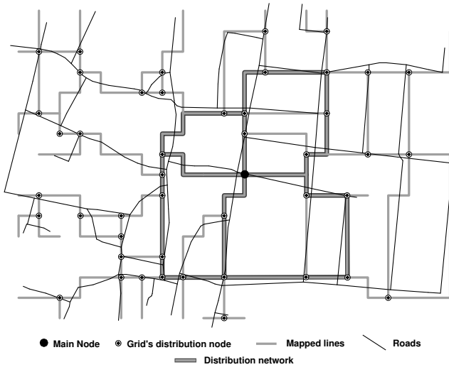
Figure 4. Including distribution network in Grid network.
